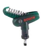
10-piece "Pocket" screwdriver bit set 9 screwdriver bits L = 25 mm PH 1/2, PZ 1/2/3, HEX 4 / 5, T 20/25 1 hand screwdriver, ratchet function clockwise/ counterclockwise
