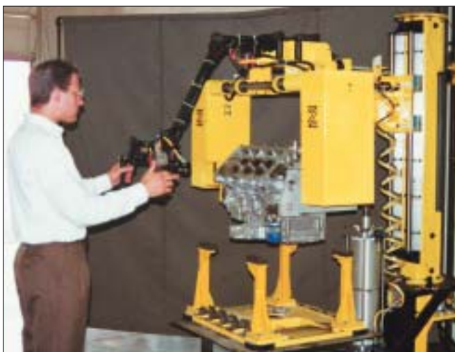
Air clamp handling device for engine rollover
