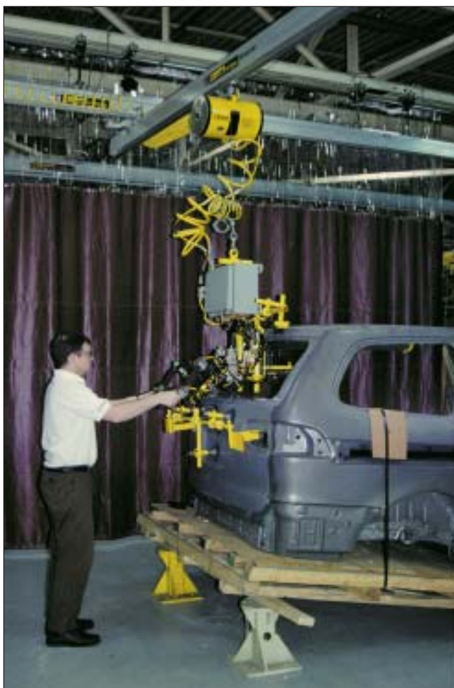
Vacuum end effector integrated with 4 Ingersoll-Rand D-Series nut runners shown installing a lift gate assembly.
